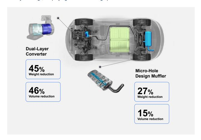
Together with thinner-gauge stainless steel, LeanExhaust's innovations contribute to a 15.6 kg weight reduction compared to conventional exhaust systems, while exceeding or matching emissions-control and noise-reduction performance.
