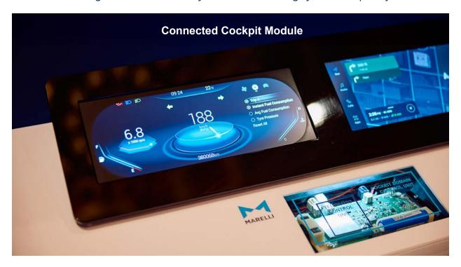
By consolidating software control of the instrument cluster, IVI and 4G telematics into one control unit powered by a single SoC, LeanConnect replaces three separate ECUs with one. This unique integration eliminates duplication of the MCU and the associated engineering effort in one simplified package.
