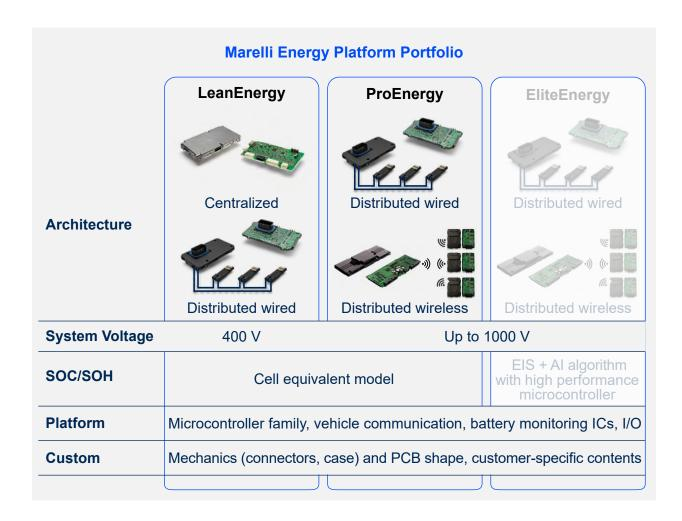
Marelli's approach leverages modular design principles, where foundational components such as the main MCU, communication lines and battery-monitoring integrated circuits are shared across platforms, ensuring consistency and efficiency. Meanwhile, mechanical components are crafted to remain bespoke, enabling customization that aligns with OEM-specific integration requirements.
