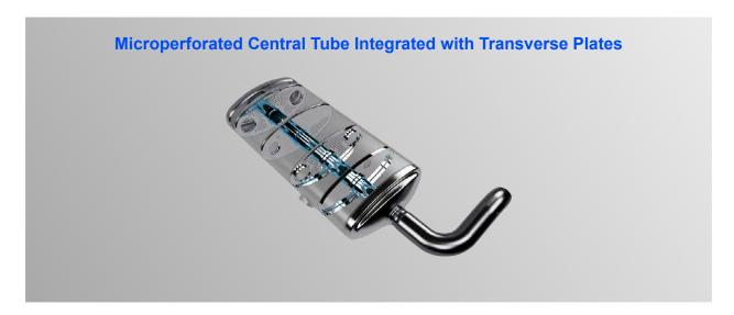
This promotes air-particle vibration inside the muffler casing, converts exhaust gas energy into thermal energy and suppresses exhaust sound.
