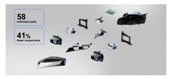
Overall, simplification reduces average production cycle times by 16% and cuts assembly effort by 20%.
