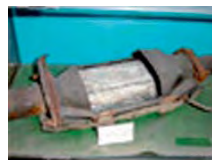
Used catalysts for purifying exhaust gases
