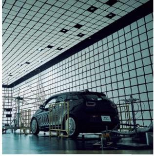
EMC Test, a type of verification test at the "vehicle" stage of the Quality Assurance Process (right)
