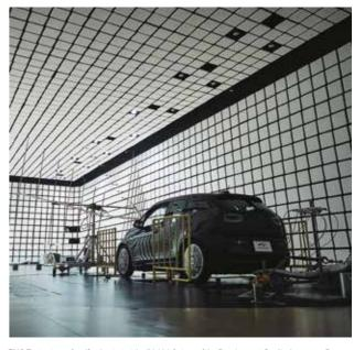
EMC Test, a type of verification test at the "Vehicle" stage of the Development Quality Assurance Process
