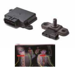
Above: Current weight detection type ODS. Below: Next generation ODS that distinguishes between adults and children using a unique algorithm based on the skeleton of the occupant detected in a near-infrared camera image. The next generation ODS is capable of supporting airbag deployment control as well as individual authentication making it possible to reproduce the occupant's desired air conditioner and other settings.
