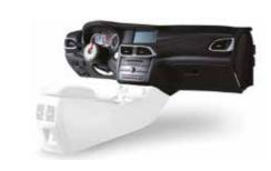
Achieved a weight reduction of 35% in the cross-car beam by changing to aluminum and 30% in the instrument panel lining with the use of foam molding
