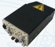
The dc-dc converter generates low voltage (12V and 48V) power for the car's electrical systems from the high voltage hybrid power battery (900V). The converter is designed with high voltage SiC (Silicon Carbide) transistors whose high switching speed achieves 2kW power from a device weighing only 1.6kg. From a sustainability point of view, it guarantees high efficiency and lower mass and is used in hybrid vehicles.
